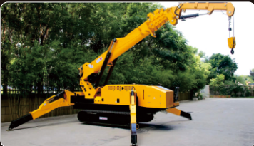
9' 10" HYDRAULIC JIB MAX LIFTING WEIGHT 1,545 lbs
